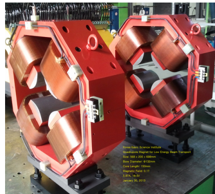
(b) Quadrupole magnet
