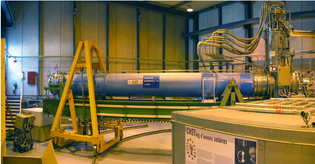
Figure 3.4: A picture of the CERN Axion Solar Telescope in the experimental Hall. The 10 m long magnet is moving with the help of a platform sitting on two ends: a turntable on the right, allowing it to move \pm 40^\circ horizontally, and a girder (left) supporting the two screws that move the magnet \pm 8^\circ vertically. The turntable holds the weight of the MFB, while the much less weight of the MRB is born by the screws. The flexible helium transfer lines were designed to allow the movement of the magnet without interrupting its cryogenic operation.
