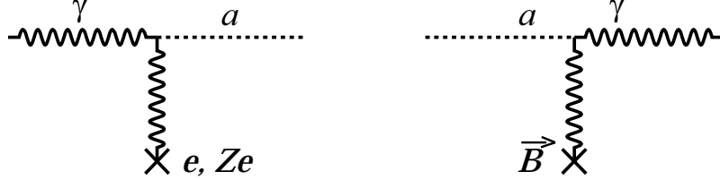
Figure 3.1: The Primakoff effect in the Sun (left) and the inverse process in the laboratory-magnet (right).
