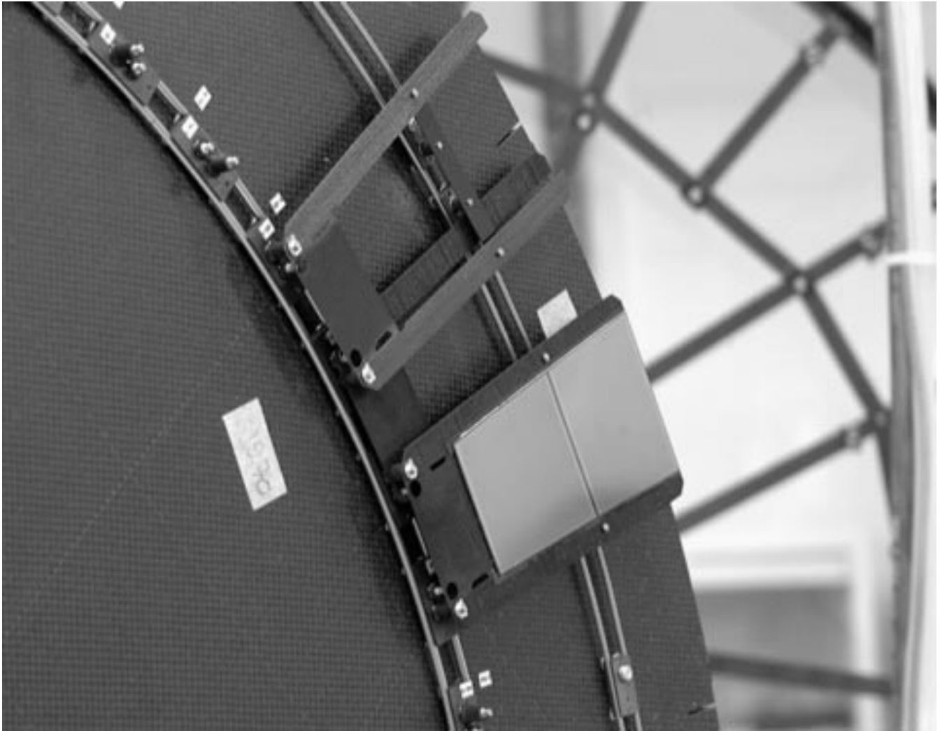
Figure 22: View of a prototype support structure for an inner forward disk, one dummy silicon module is mounted.
