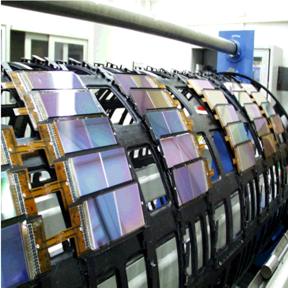
Figure 21: View of a prototype support structure for the inner barrel, some dummy silicon modules are mounted.
