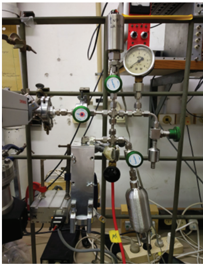
Figure 2. Manifold used for the dilution of the irradiated Ar-gas with ^{nat}\text{Ar} . The ILL1 sample cylinder is at the right-hand end of the vacuum line.
