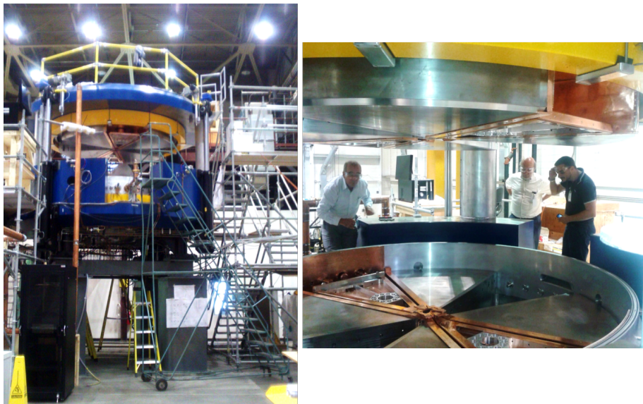
Fig. 1. The main magnet of the cyclotron lodging the tested RF resonators.
