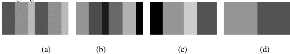
Fig. 2: (a) is a grey scale image. (b), (c), and (d) shows segmentations of the image with d=97\% , 98\% , and 99\% , respectively
