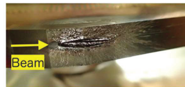
Figure 2: Collimator head damaged by SBL.
