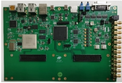
Figure 5: The prototype DSP board.
