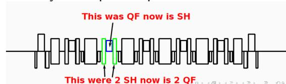
Figure 1: Change on the sextupole/quadrupole position.
