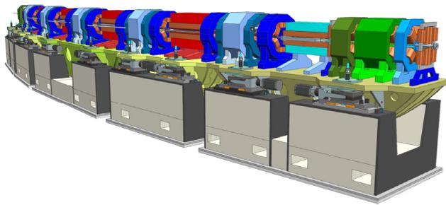
Figure 6: Girder, magnets and vacuum assembly of a cell.
