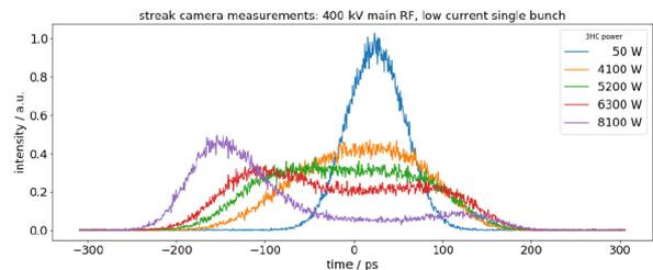
Figure 8: Bunch lengthening beam tests at BESSY II with the 3<sup>rd</sup> Harmonic EU Active Cavity Prototype.
