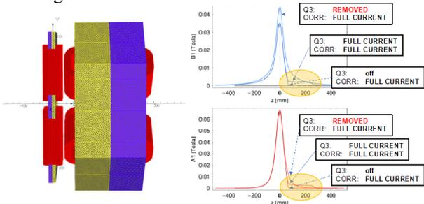
Figure 4: Corrector and Q3 separated by 55 mm yoke to yoke; and magnetic cross-talk.
