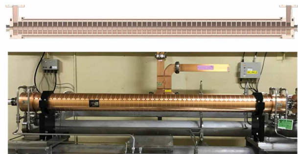
Figure 1: Cut-off schematics (Upper) and the structure installed in the injector tunnel (Lower).
