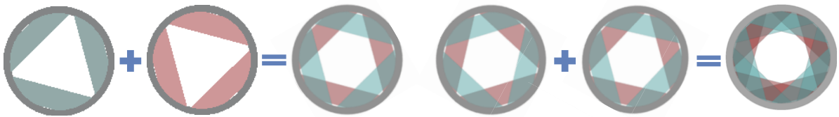
Figure 3. Assembly of a tracker station. Six panels of 96 groups of straws are assembled into a panel. Two panels form a tracker station.
