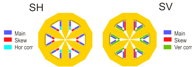
Figure 2: Proposed configuration of coils for horizontal and vertical sextupoles for ALBA II.
