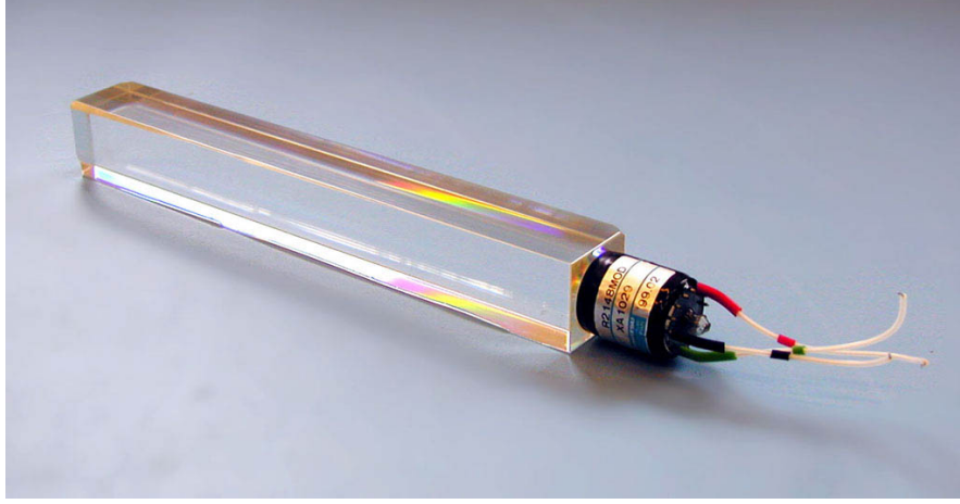
Figure 3.4: An endcap \text{PbWO}_4 crystal with a phototriode attached.
