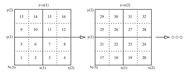
Figure J-1. Superimposed mesh cell indexing
