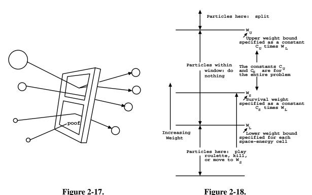
Figure 2.18 is a more detailed picture of the weight window. Three important weights define the weight window in a space-energy cell
