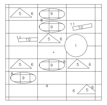
This example illustrates a more complicated lattice geometry and uses the FILL card followed by the array specification. It builds on the expertise from example 4. There are three "main" cells: cell 1 is inside surface 5, cell 3 is the outside world, and cell 2 is the large square (excluding cell 1) that is filled with a lattice, some of whose elements are filled with 3 different universes.
