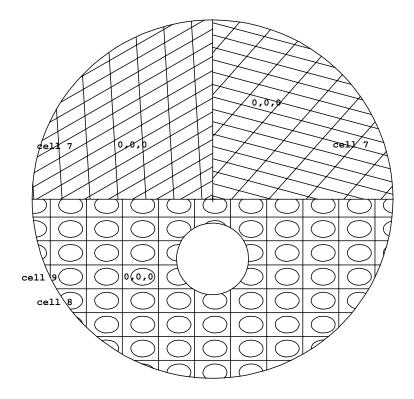
This example illustrates a lattice geometry and uses the FILL entries followed by transformations, the U card, and the LAT card. Cell 2 is the bottom half of the large sphere outside the small sphere (cell 1), is filled by universe 1, and the transformation between the filled cell and the filling universe immediately follows in parentheses.
