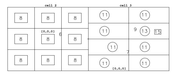
In brief, a volume distributed source located in each of the ten boxes and eight circles (in two dimensions) is desired. The cells involved are given by distribution 6. The S on the SI6 card indicates distribution numbers will follow. The four distributions will describe the cells further. The probabilities for choosing each distribution of cells is given by the SP6 card.
