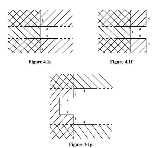
There is more than one way to define cell 3. Starting with surface 1, we can add the region to the left of 1 to the region outside surface 2 or -1: 2, which is illustrated in Figure 4.1h. We wish to intersect this space with the space having a negative sense with respect to surface 3. Superimposing
