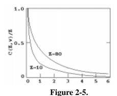
For next event estimators, one must evaluate the probability density function  $p(\mu) = \pi r_0^2 (1 + \mu^2) C^2(Z, \nu) / \sigma_2(Z, \alpha)$  for given  $\mu$ . Here  $\sigma_2(Z, \alpha)$  is the integrated coherent cross section. The value of  $C^2(Z, \nu)$  at  $\nu = \kappa \alpha \sqrt{1 - \mu}$  must be interpolated in the original  $C^2(Z, \nu_i)$  tables separately stored on the cross-section library for this purpose.
