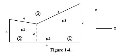
With surface 6 added to Figure 1.4, the cell to the right of surface 6 is number~1 (cells indicated by circled numbers); to the left number 2; and the outside cell number 3. The cell cards (in two dimensions, all cells void) are
