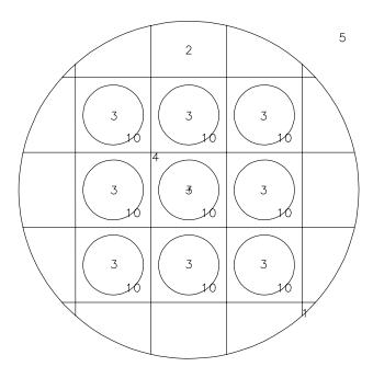
This is a simple example illustrating the use of the FILL, U, and LAT cards to create an object within several cells of a lattice. A hexahedral lattice is contained within a cylinder of radius 45 cm. Cell 1 is the interior of the cylinder, and cell 5 is everything outside (all surfaces are infinite in the z-direction). Cell 1 is filled by universe 1. Cell 2 is defined to be in universe 1. Surfaces 301-304 define the dimensions of the square lattice.
