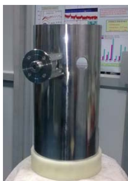
Fig. 7b, c Integrated assembly of Collimator, beam scanner & electron capture electrode ( 180^\circ views)
