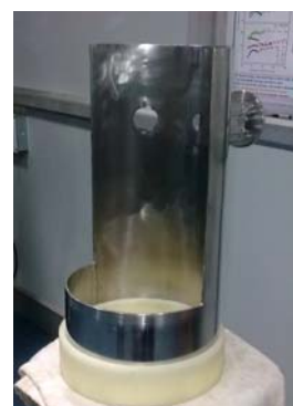
Fig. 7b, c Integrated assembly of Collimator, beam scanner & electron capture electrode ( 180^\circ views)
