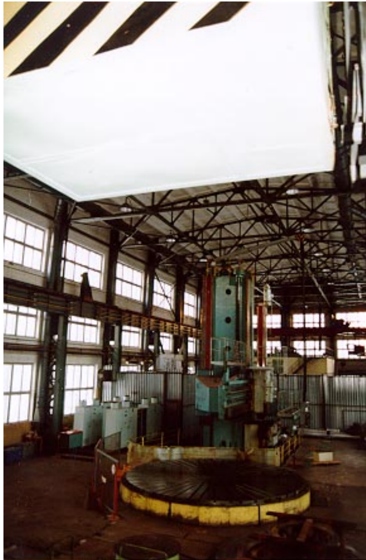
Figure 3-6. The largest milling machine of the JINR workshop. The diameter of the rotating table is expandable up to 14 m.
