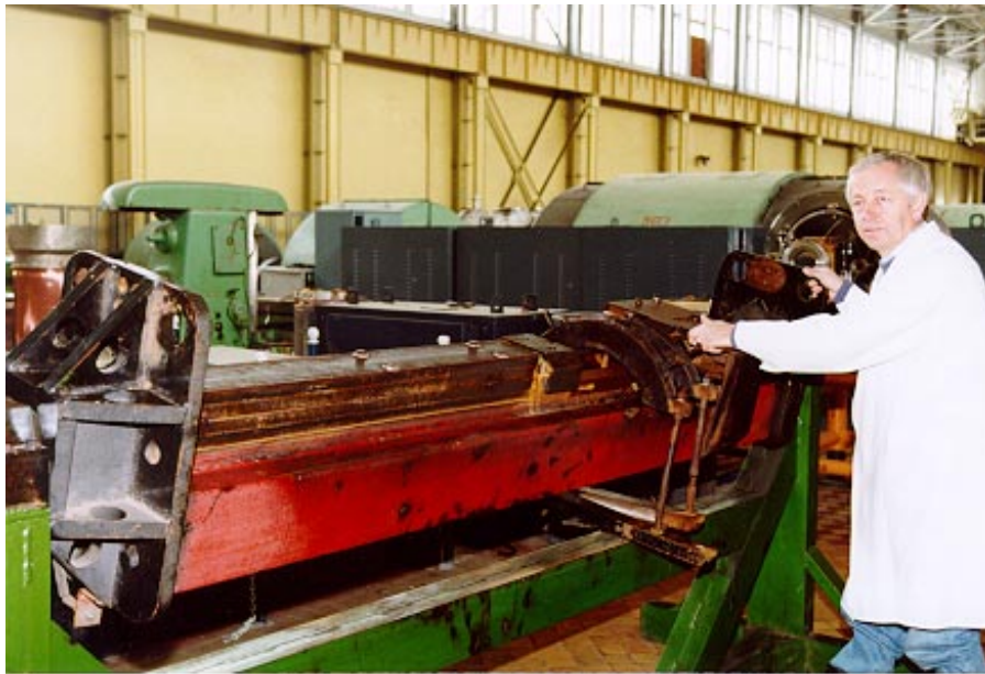
Figure A3-1. The winding device that could be adapted to wind the coil model in 1:3 scale.
