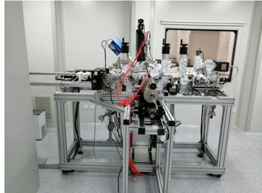
Figure 1: Photocathode preparation device.
