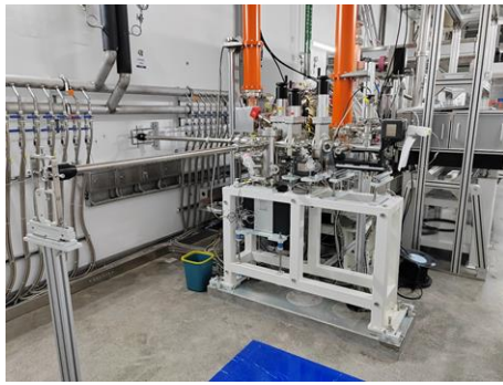
Figure 8: Photocathode loading device and VHF electron gun.
