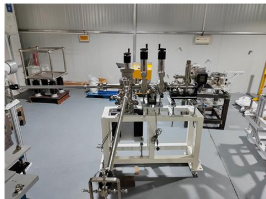
Figure 2: Photocathode loading device.
