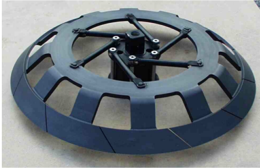
Figure 4.9: A picture of the actual Target E. Each of the twelve segments is separated by a 1 mm gap to allow for thermal expansion and deformations.
