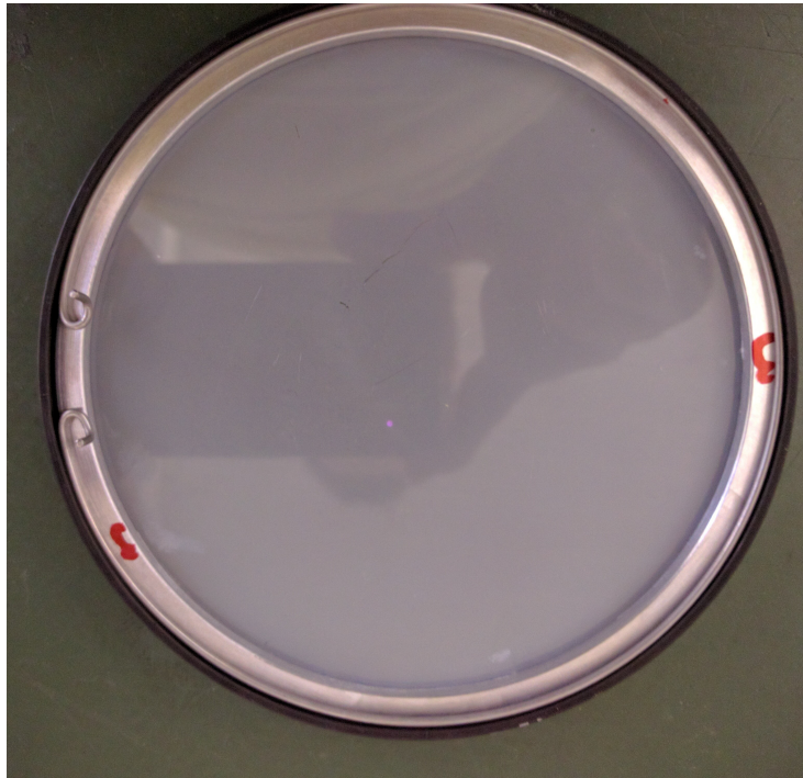
Figure 6.4: One of the CsI(Tl) luminophore foils used in the muon beam test with a CsI(Tl) layer thickness of 5.2\mu\text{m} on a 3\mu\text{m} MYLAR substrate. The foil diameter is 125 mm.
