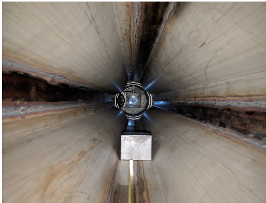
(a) A picture of the positron-stopper inside the cross-shaped vacuum chamber of TII in the gap between QSK41 and QSK42.
