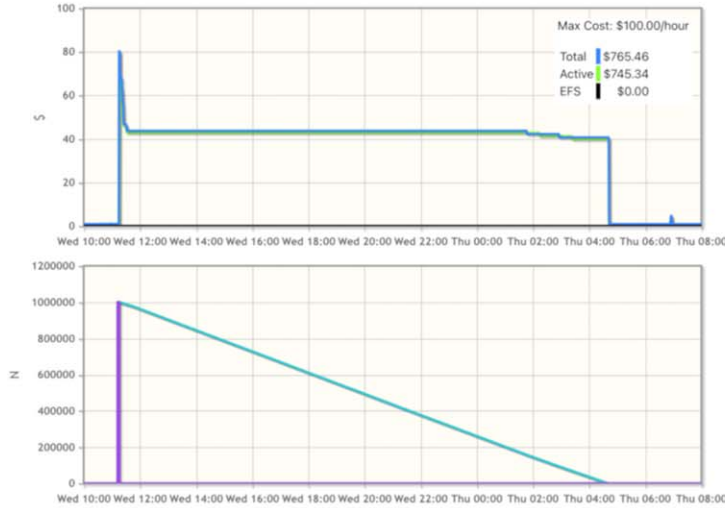
Figure 1. FNC data handling. Top left: a summary view of the workload, generated by FNC. FNC handled 1 million jobs corresponding to the computation of each individual spectrum for a total compute time of 1 yr and 66 days, performed in only 17 hr and a half. Bottom left: the top graph shows the total cost incurred for this computation as a function of time. The bottom graph shows the jobs queued waiting to be executed. Right: report showing the workload, for convenience broken down into 40 sets of 25,000 jobs each. Notice that 45 jobs have been labeled as failed after the first computation, due to the interruption of spot instances. FNC allows effortless rescheduling of those 45 failed jobs, and within a few minutes all jobs were done.
