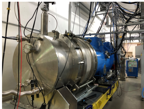
Figure 2: 3.9 GHz small cryomodule under horizontal test.
