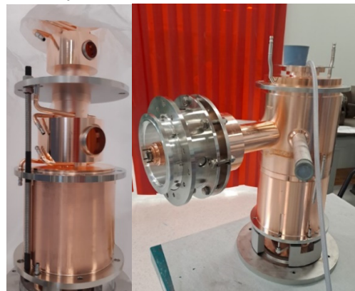
Figure 7: Picture of the cavity subassemblies: Left: cavities 2,3 and 4. Right: penultimate and output cavity.
