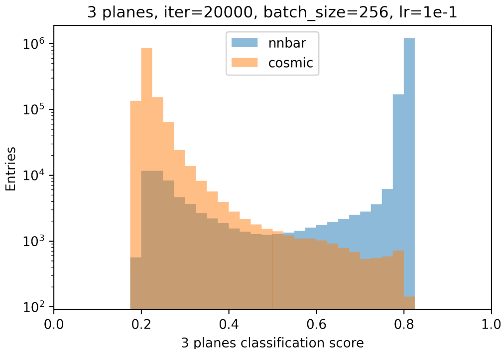
Figure 7.19: CNN signal score distribution for n - \bar{n} and cosmic clusters using CV sample. 1,633,525 n - \bar{n} clusters and 1,618,827 cosmic clusters are classified by the trained CNN classifier.
