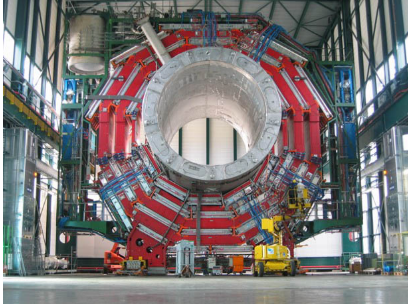
Figure 3.9: Picture of the CMS solenoid magnet together one of the barrel yoke “wheels”.
