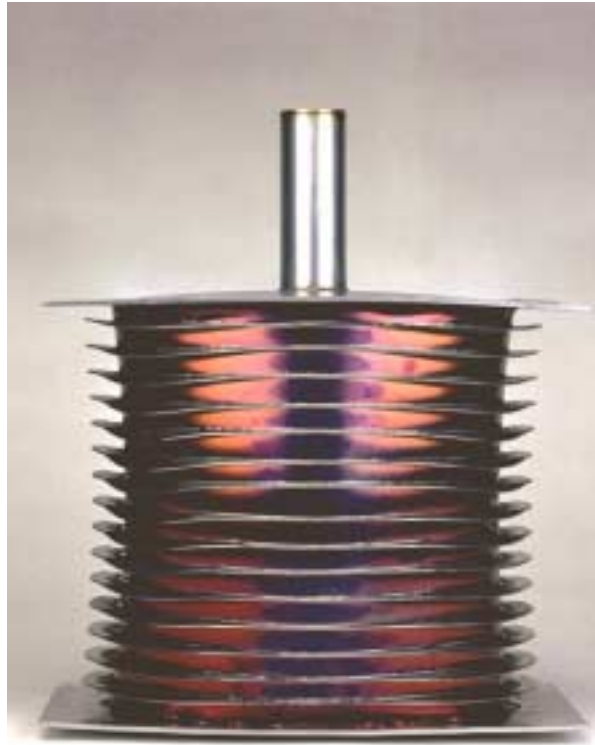
Figure 8.9. Photograph of Unsuccessful Prototype of Rib-Reinforced Vacuum Chamber
