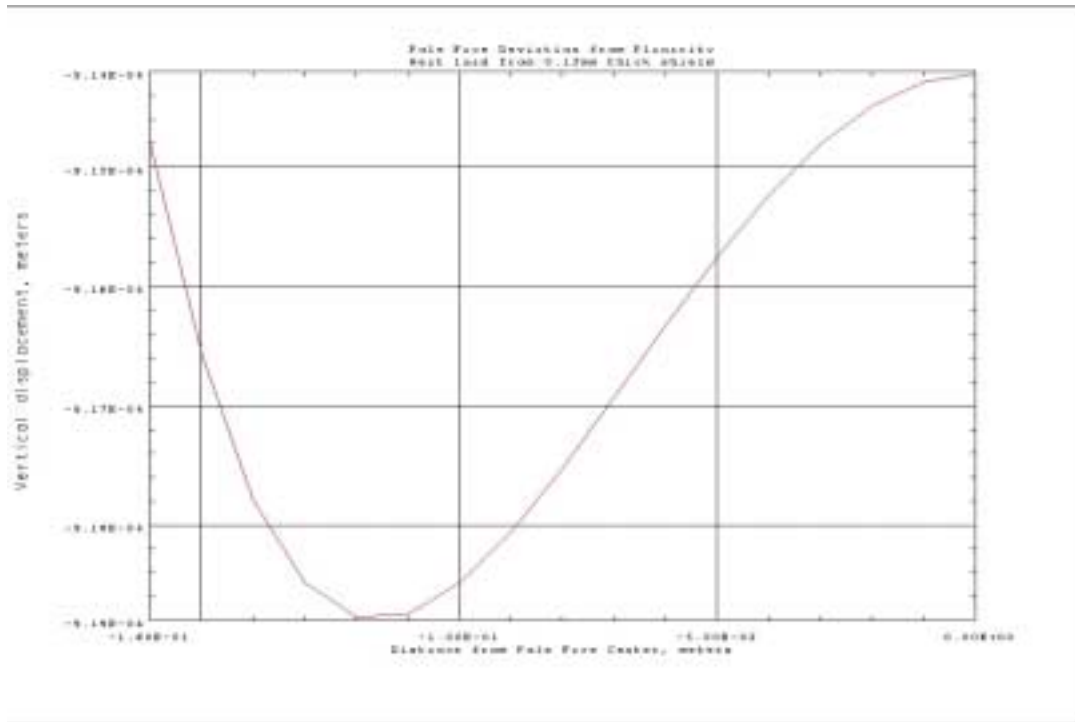
Figure 8.7. Plot of Vertical Component of Dipole Pole Face Thermal Displacement
