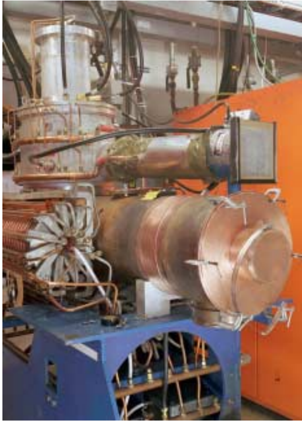
Figure 5.10. Booster cavity with ferrite tuner in foreground
