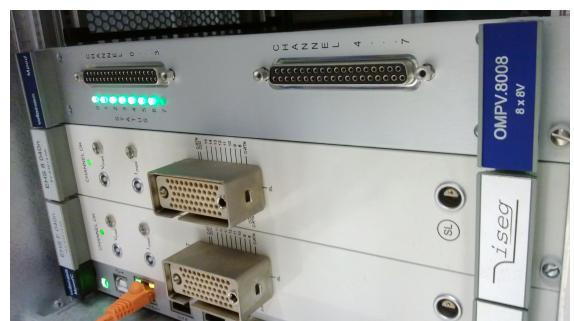
(b) Wiener crate with a low-voltage and two high-voltage modules.
