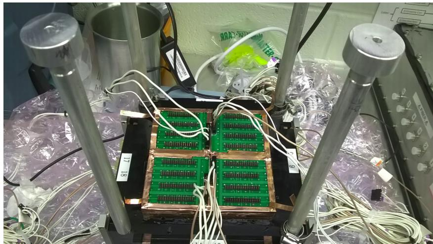
(b) Copper frame mounted on the bottom face (during the electronics swap).
