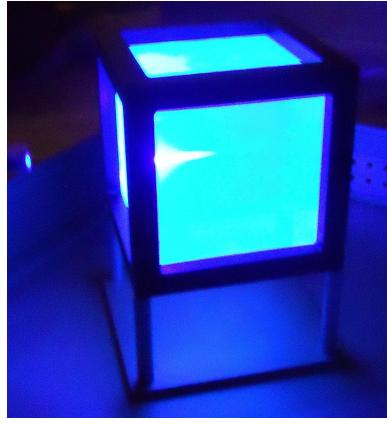
(a) mTC scintillator illuminated by a blue laser.
