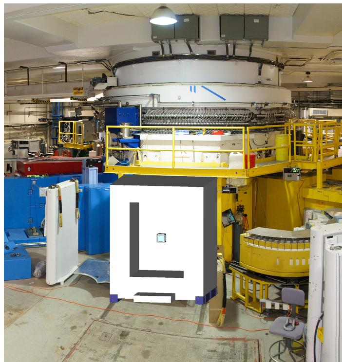
Figure 2.132: Photograph of the location next to the reactor with a diagram of the mTC cave and the scintillator cube added.
