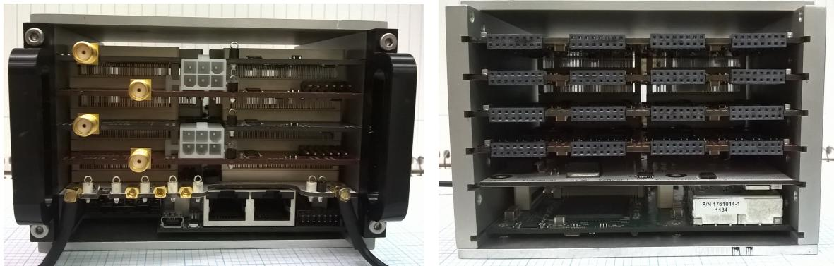
Figure 2.61: Left: Back of one of the twelve board stacks. LV (2 molex connectors), JTAG and clock (2 RJ-45 connectors), fiber optic interface.
