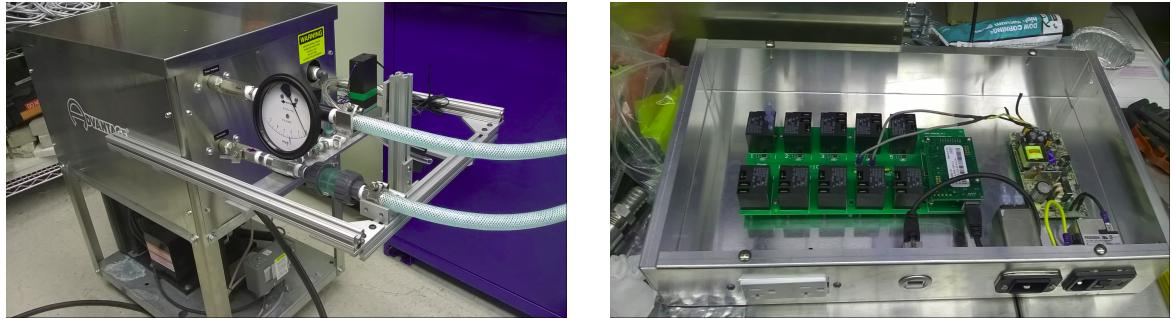
(a) Chiller with analog flowmeter, pressure release valve, and coarse filter.
