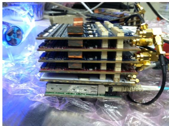
(a) 4 copper heat sinks each covering 4 chips installed in a readout module.
