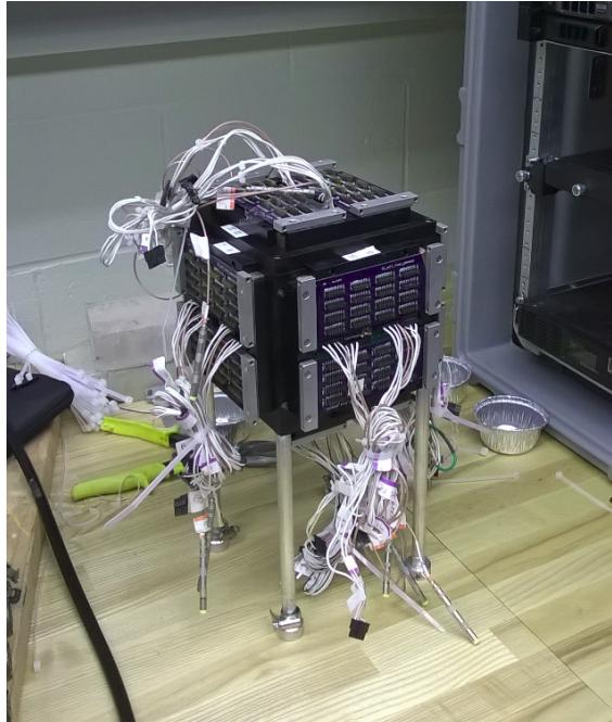
(a) MCP-PMT with front boards attached on each face of the mTC.
