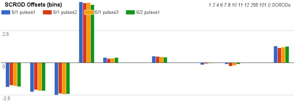
Figure 2.32: Timing offsets. Four timing-groups among 12 board stacks for different function generator calibration runs. The data were taken using a pulser with the following parameters: 2.6Vpp, 1.5kHz, 8ns width, 5ns rise/fall, no offset; the pulser signal was fed through a 12-way power splitter to each SCROD calibration input. In reality, one bin corresponds to  $\sim .3\text{--}.4$  ns. Figure is taken from [88].
