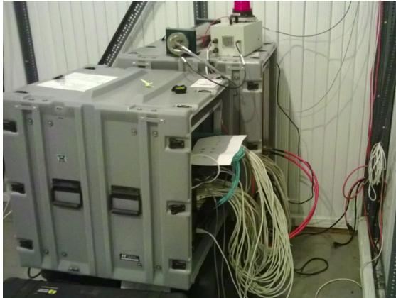
(a) Deuterium-tritium 14-MeV neutron generator (Thermo Scientific P 385) on top of mTC main crate. Spring 2014.
