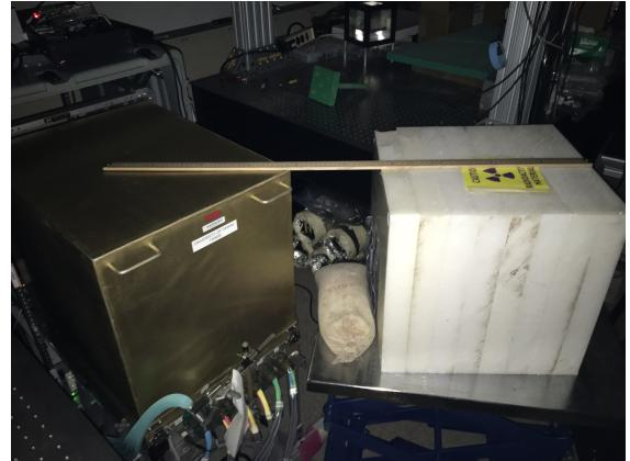
(b)  $^{252}\text{Cf}$  in the white poly shield is located on an adjustable platform, next to the mTC. Spring 2017.
