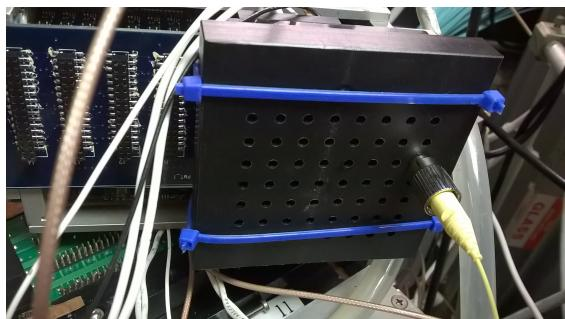
(a) MCP-PMT pincusion test with one fiber illuminating edge pixels.
