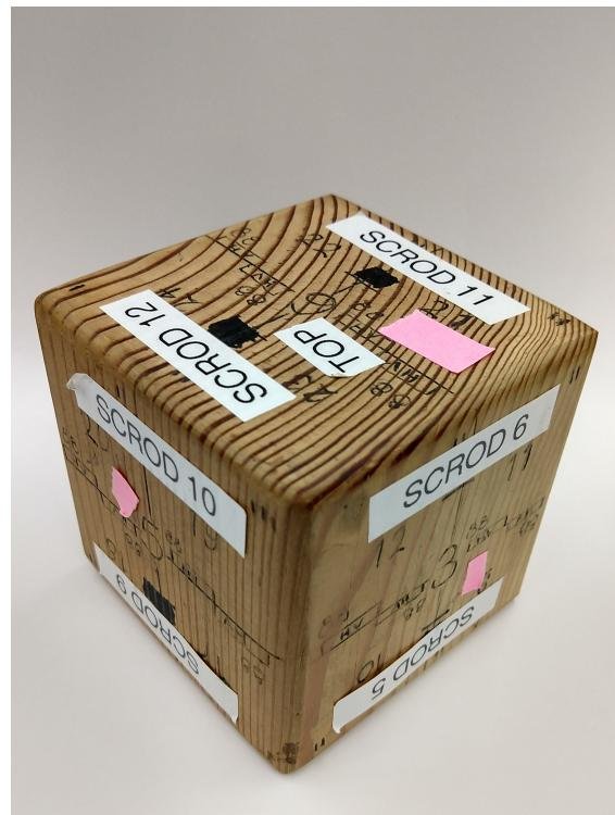
(b) Wooden model of the cube indicating the locations of the PMTs and readout modules.
