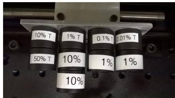
(b) Neutral density filter slide, adjusting light output to single-PE level.
