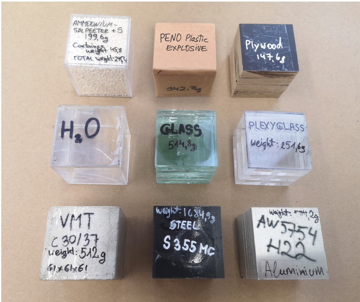
Figure 5. The test samples used for this exercise. Starting from the top left, moving left-to-right and top-to-bottom: ammonium nitrate with sulphur pellets, PENO plastic explosive, plywood, water, glass, plexiglass, concrete, steel, and aluminium.
