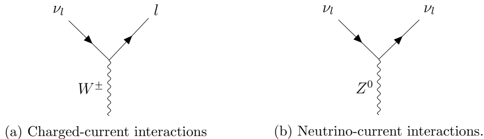
FIGURE 1.1: Feynman diagrams of neutrino interactions in the Standard Model. (a) Feynman diagram vertex for charged-current interactions where a neutrino changes to a charged lepton (or vice versa) via the exchange of the W^\pm vector boson with another particle. (b) Feynman diagram vertex for neutral-current interactions where a neutrino interacts via the exchanges of the Z^0 vector boson.
