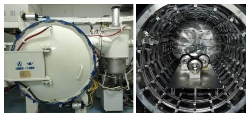
Figure 1: High temperature furnace for cavities annealing and three single cell cavities in the chamber before annealing.
