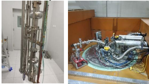
Figure 3a: Two single cell cavities were assembled together. 3b: Vertical test system at Peking University.
