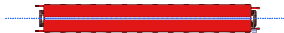
(a) Top view of the SPS dipole magnet. Blue dots indicate scan positions along the longitudinal z -axis.
