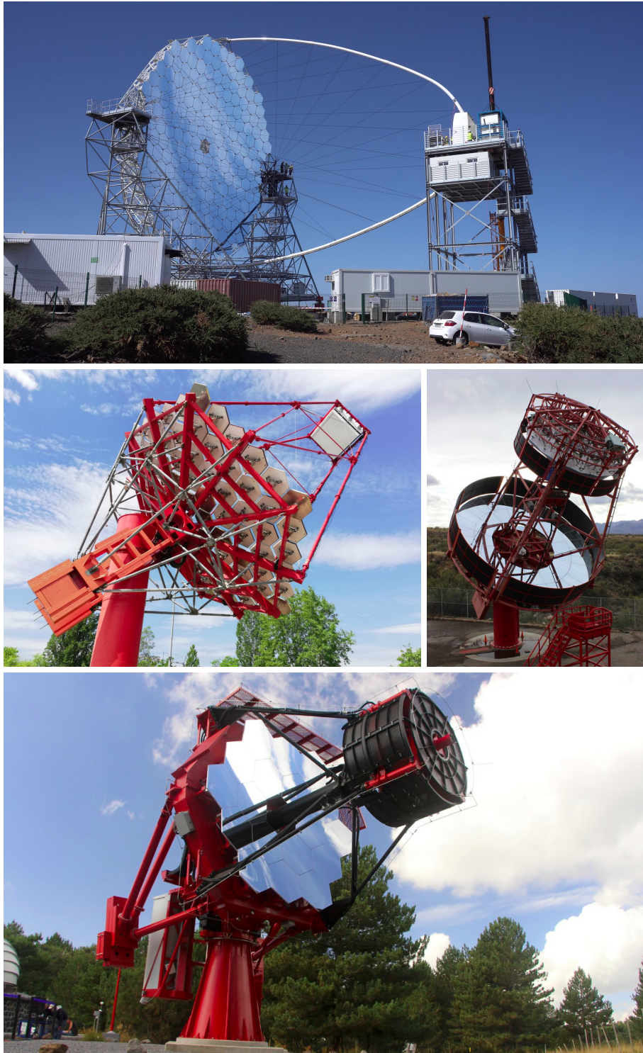
Figure 26 – Prototypes of CTA telescopes. Top: the large-size telescope. Middle left: the Davies-Cotton designed mid-sized telescope. Middle right: the dual mirror Schwarzschild-Couder mid-sized telescope. Bottom: the dual mirror Schwarzschild-Couder small sized telescope.
