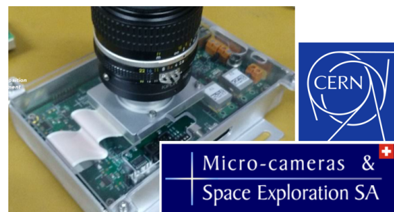
Figure 2: Picture of the ‘BeamCam’ camera prototype ready for the irradiation test.
