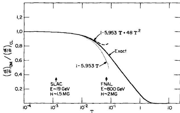
Fig. 3 Ratio of QM and CL radiation rates
