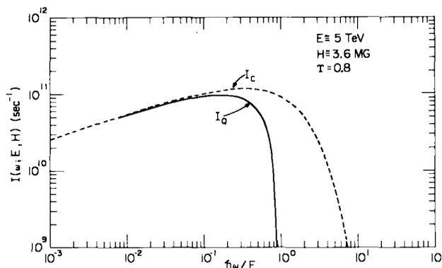
Fig. 1 Comparison of classical and quantum mechanical synchrotron spectra
