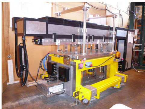
Figure 1. Photo of one set of ZDC calorimeters on the movable platform on the surface.
