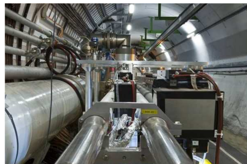
Figure 2. Photo of one set of ZDC calorimeters on the movable platform in the tunnel.
