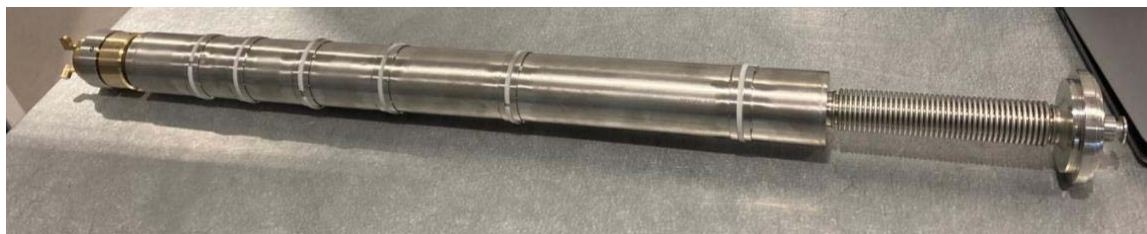
Figure 9. VLP return valve insert with wipers as convection brakes against TAO
