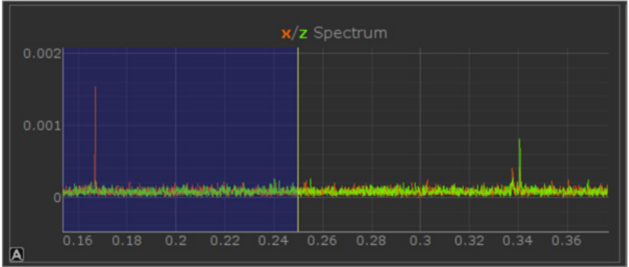
Figure 12: Coherent beam-beam oscillations spectrum at 479 MeV. The vertical axis corresponds to oscillation harmonic amplitude (mm).
