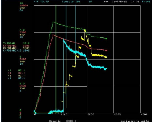
Figure 5: A typical plot of the collider ‘shot’ shows significant beam losses early in Run II (2002).
