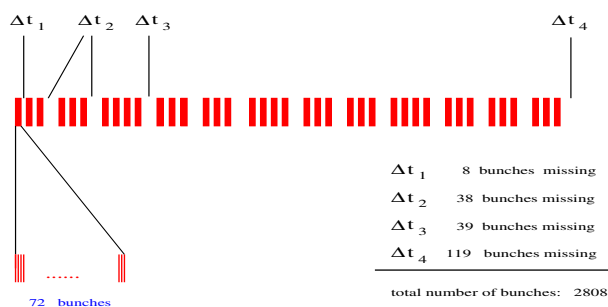
Figure 2: Bunch filling scheme of the nominal LHC.
