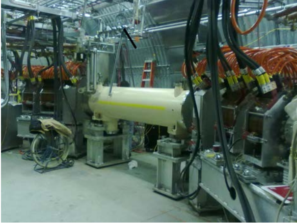
Figure 10: Yellow electron lens as installed in 2013. Visible are the gun side (left), the superconducting main solenoid (centre), and the collector side (right).
