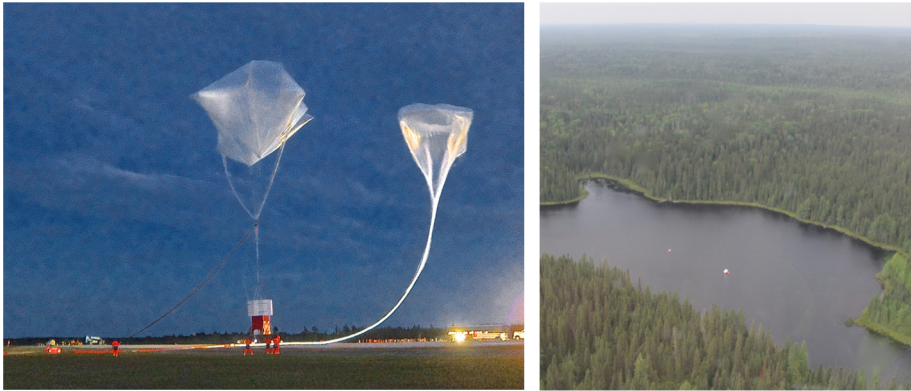
Fig. 7 Left: Timmins (Ontario, Canada) Stratospheric Balloon Base, August 25, 2014, 0:53 UTC: the perfect launch of EUSO-Balloon by the balloon division of the French Space Agency CNES, the auxiliary balloons (above the payload in the picture) warrant a smooth launch even in case of moderate surface winds. Right: the instrument floating in the middle of “Lake Euso” after splashing down at 8:59 UTC. All systems survived the impact and more than eight hours in the water thanks to a dedicated “water-landing” design
