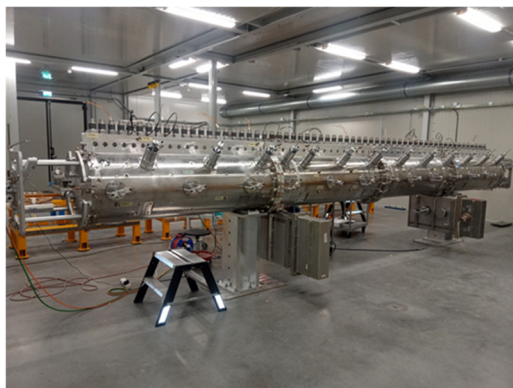
Figure 1: DTL1 on the bead pull station at ESS Lund.
