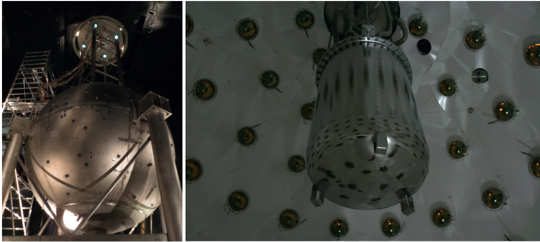
Fig. 2. Left: the borated-liquid-scintillator neutron veto. Right: the DS-50 TPC cryostat in the neutron veto.
