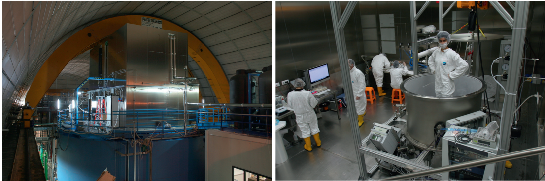
Fig. 3. Left: the water Cherenkov muon veto (blue tank) and assembly/installation cleanroom (silver box). Right: the parts-preparation cleanroom.
