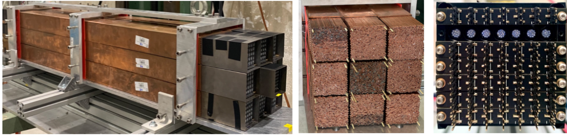
Figure 6. Left and middle: the assembled FoCal-H prototype as a matrix of 3 \times 3 modules. Right: the SiPM PCB holders attached to the central module, which comprises 7 \times 7 channels, with one PCB removed to show the fiber bundles.
