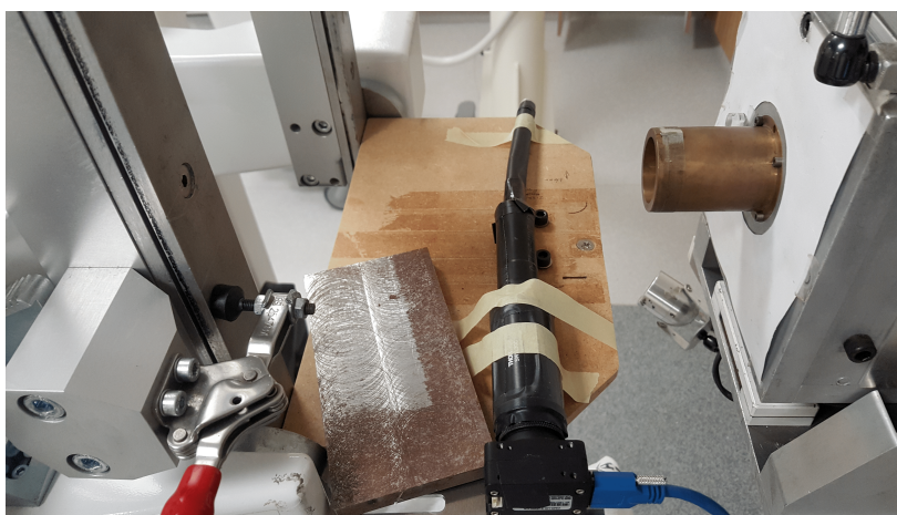
Figure 8.13: Setup of the fibre bundle positioned near the beam nozzle on the right.
