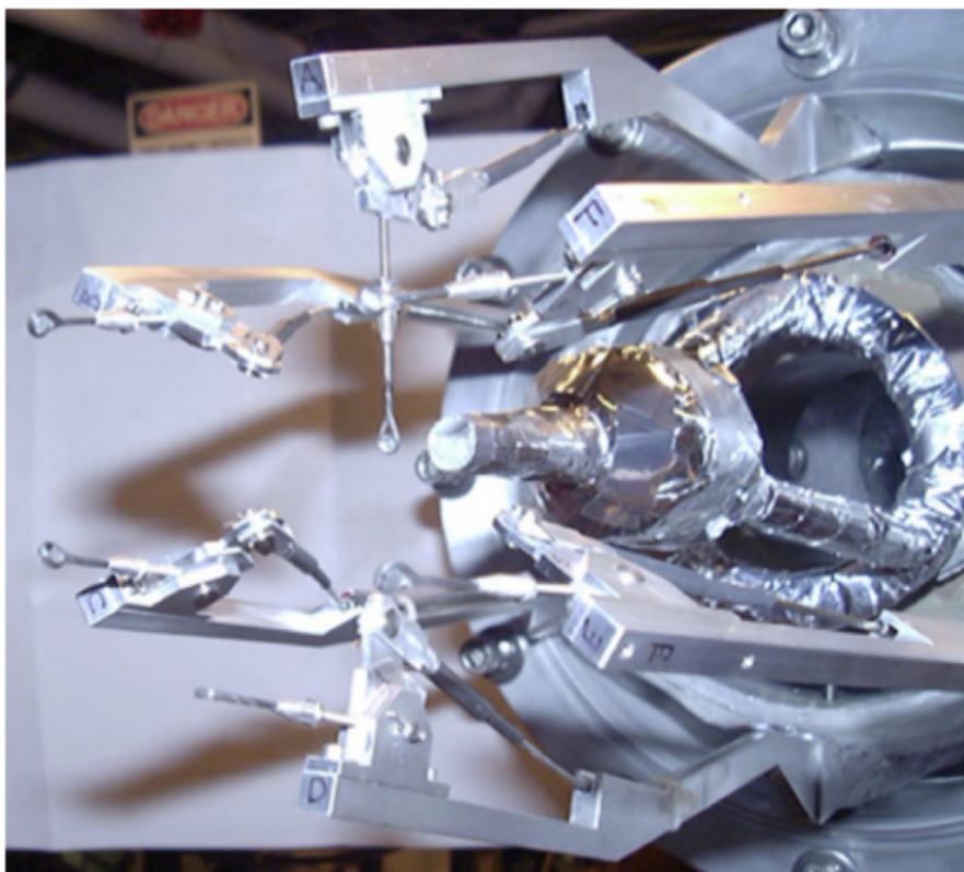
Figure 2.9: The full double-target assembly, which shows one solid target flipped on position; five solid targets retracted; and the thermally insulated cryotarget cell.
