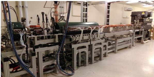
Figure 2: The NSRRC 2998 MHz photoinjector system.
