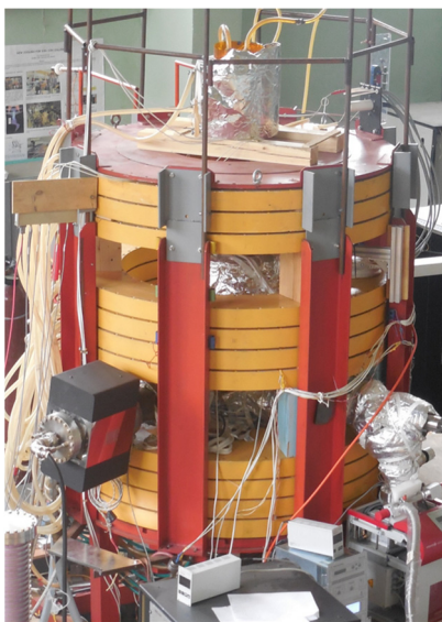
Figure 5: Test bench for electron gun.
