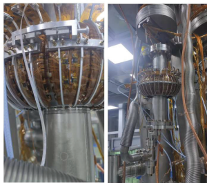
Figure 9: A T-Mapping diagnostic system is installed in a single cell superconducting cavity.
