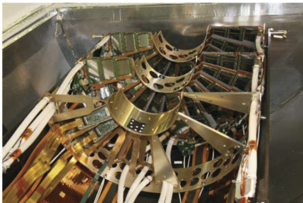
Figure 8: The pilot blade detector together with current FPIX modules that will be installed in CMS during LS1.
