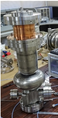
Figure 2: Prototype HOM absorber was connected with the single-cell cavity for RF measurements at room temperature.
