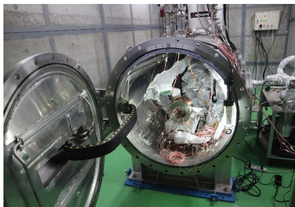
Figure 7: The prototype HOM absorber was installed in the horizontal cryostat.
