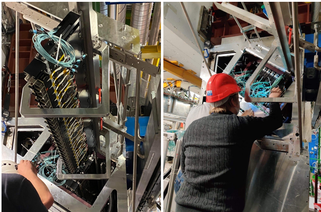
Figure 3.6: Installation of the columns in the RICH1 detector.
