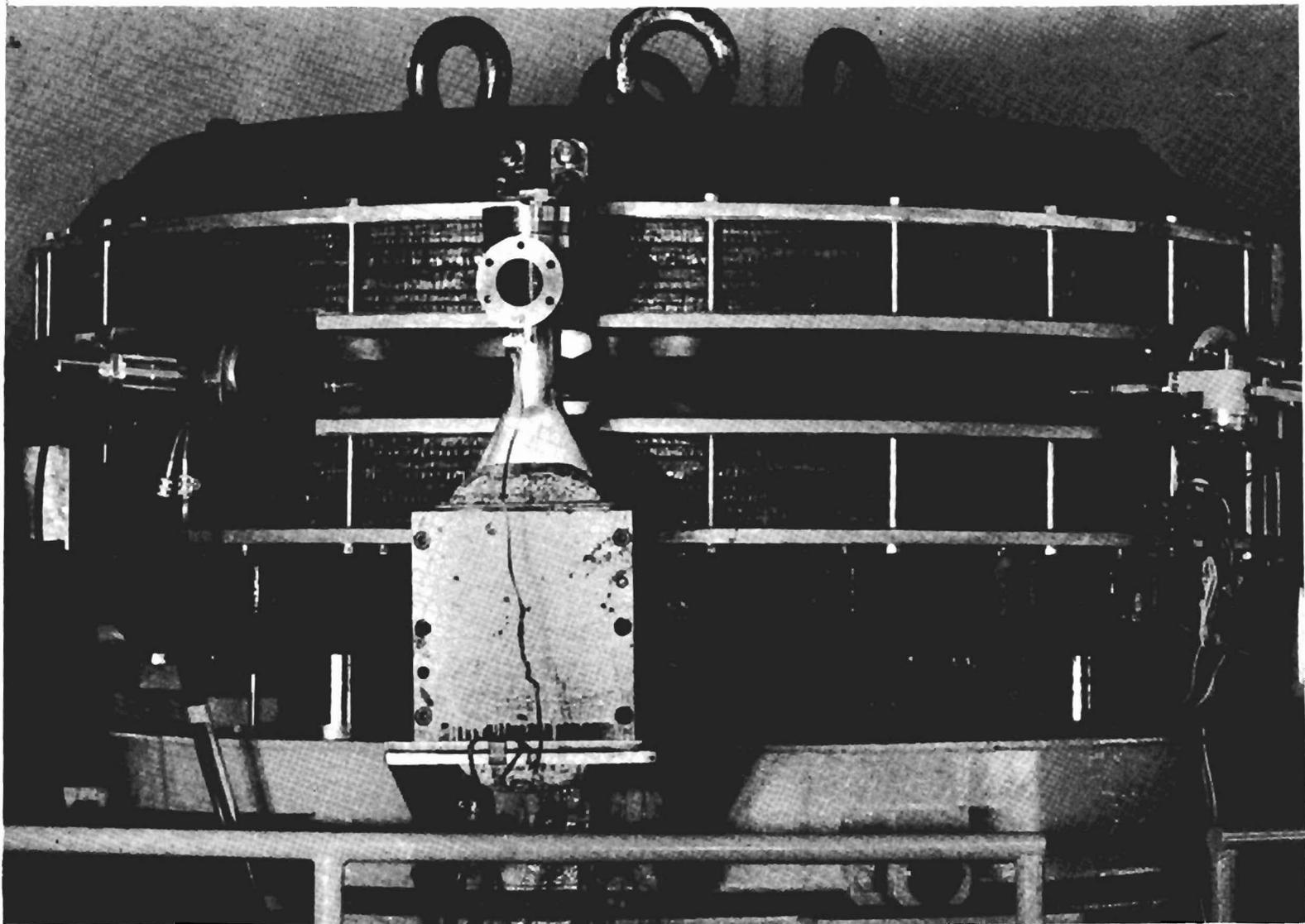
Fig. 3 - Storage ring assembled for first tests. The titanium pump is located near the center of the picture, the rf cavity to the left and target port on the right.
