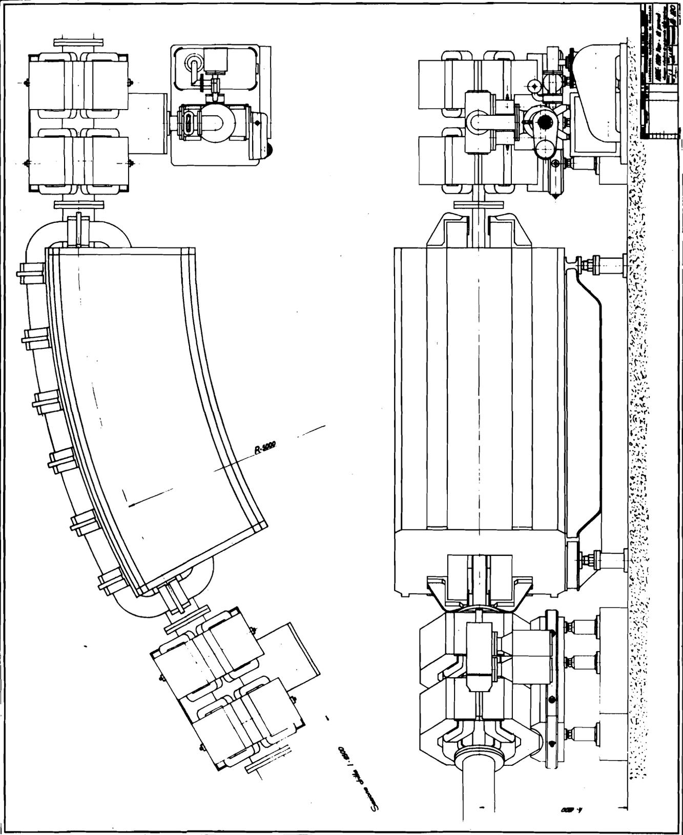
Fig. 16 - Details of Adone bending magnets and quadrupoles
