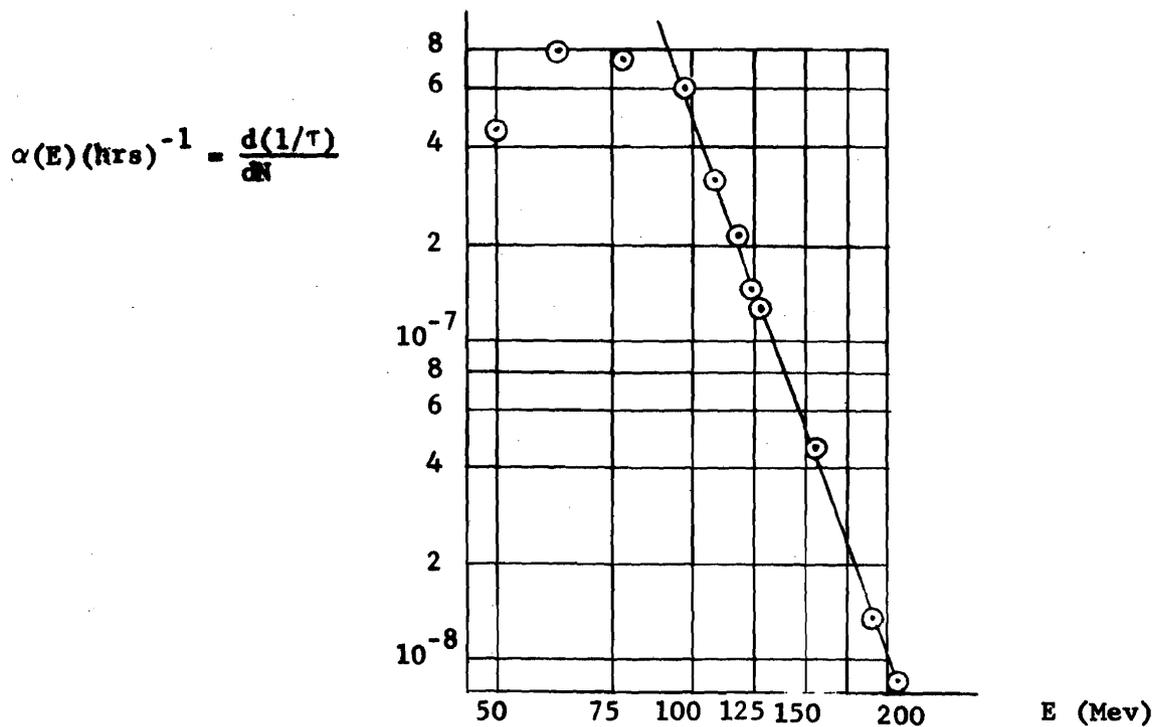
Fig. 13 - Plot of the rate  $\alpha(E)$  versus the energy of electrons in the beam
