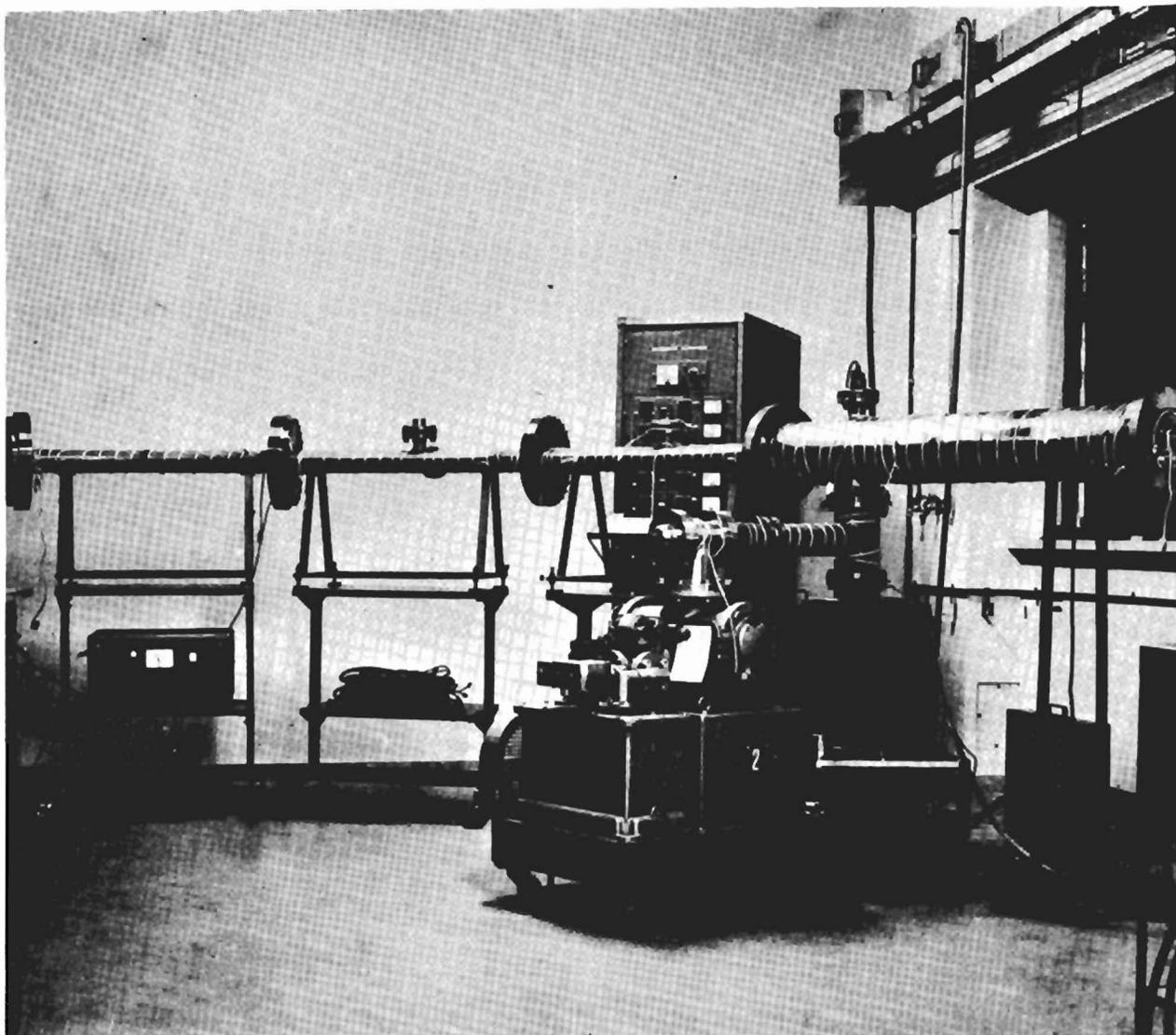
Fig. 19 - Full size model of Adone vacuum chamber. (Final vacuum flanges will be smaller than the ones shown)
