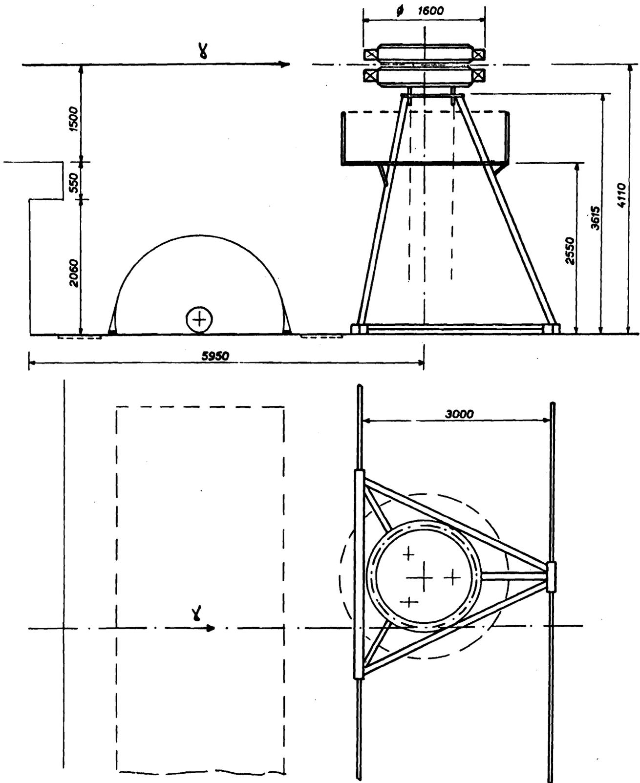
Fig. 2 - Movable tower for support of storage ring
