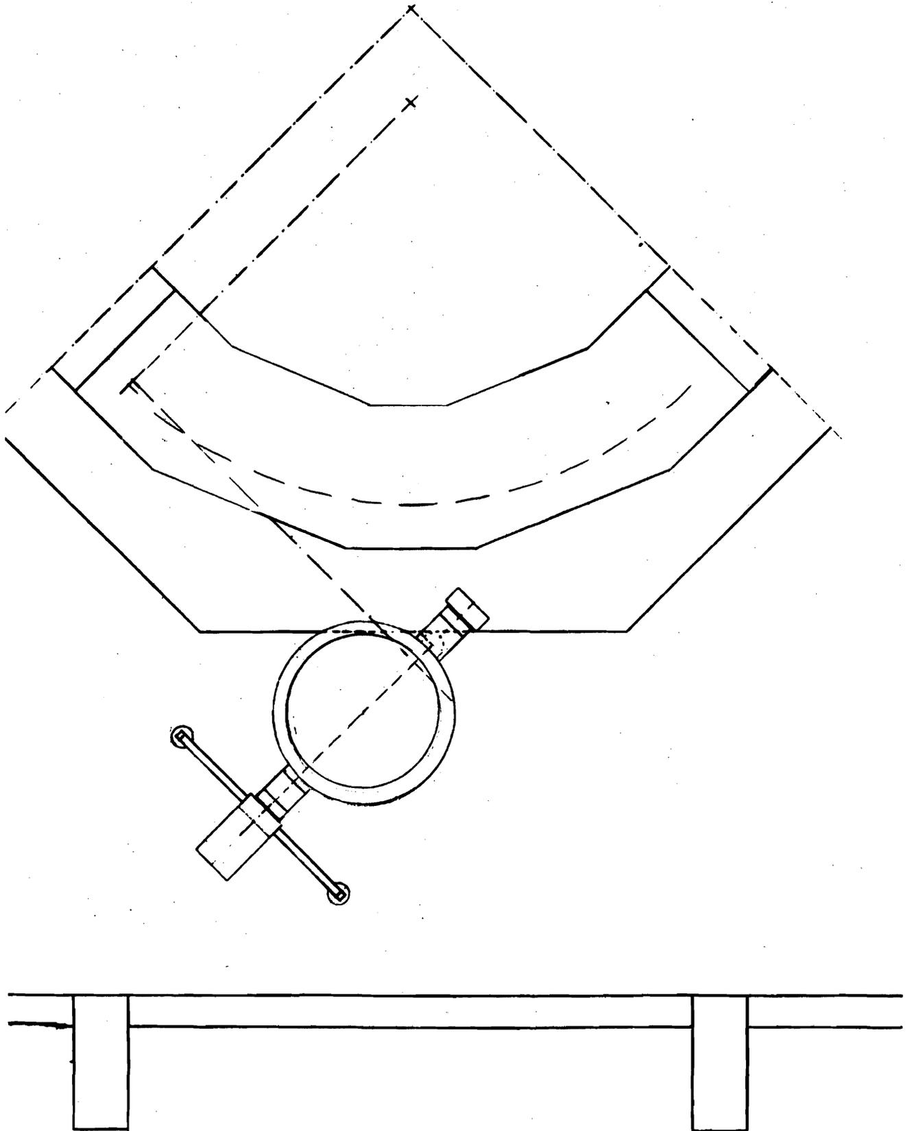
Fig. 8 - Position of storage ring after being moved closer to the synchrotron.
