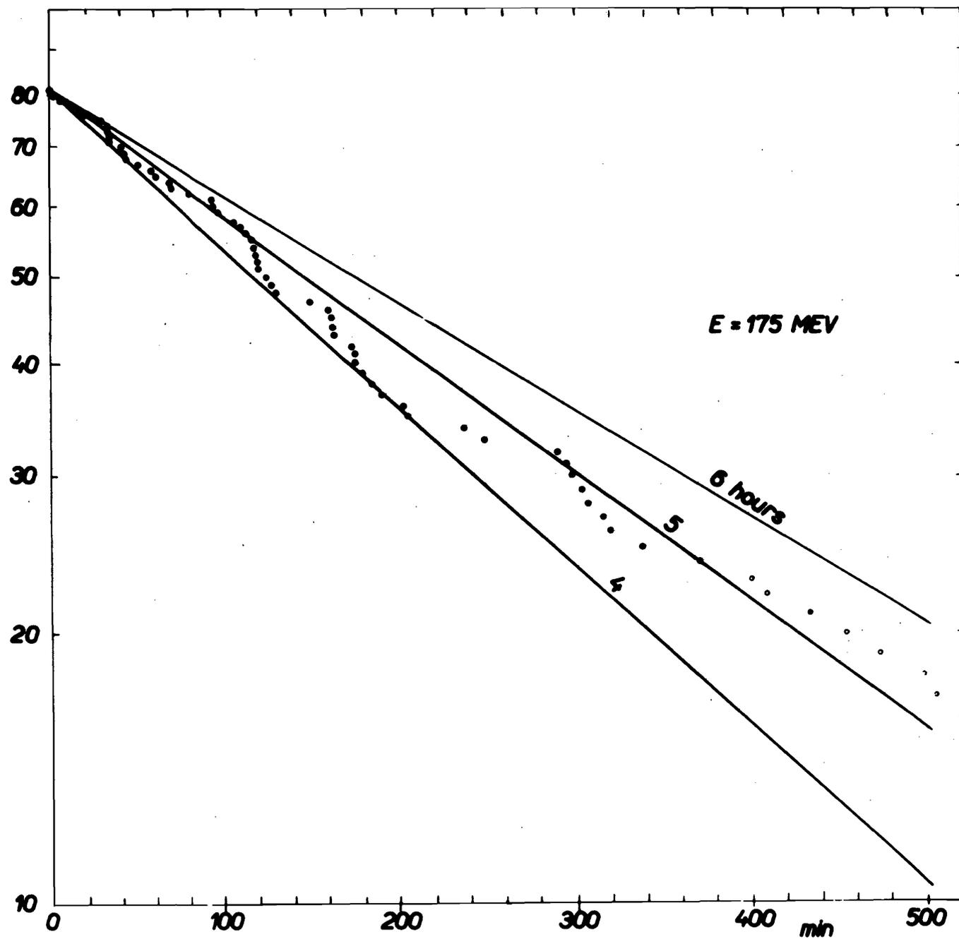
Fig. 7 - Lifetime measurement. Each dot represents the loss of one electron. Initially there were 80 electrons, pressure =  $4 \times 10^{-9}$  torr (at pump).
