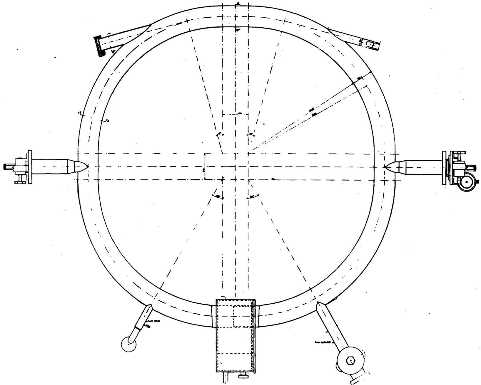
Fig. 4 - Stainless-steel vacuum chamber, showing viewing ports (top), target ports (sides), rf cavity (bottom), and vacuum ports, on either side of the rf cavity.
