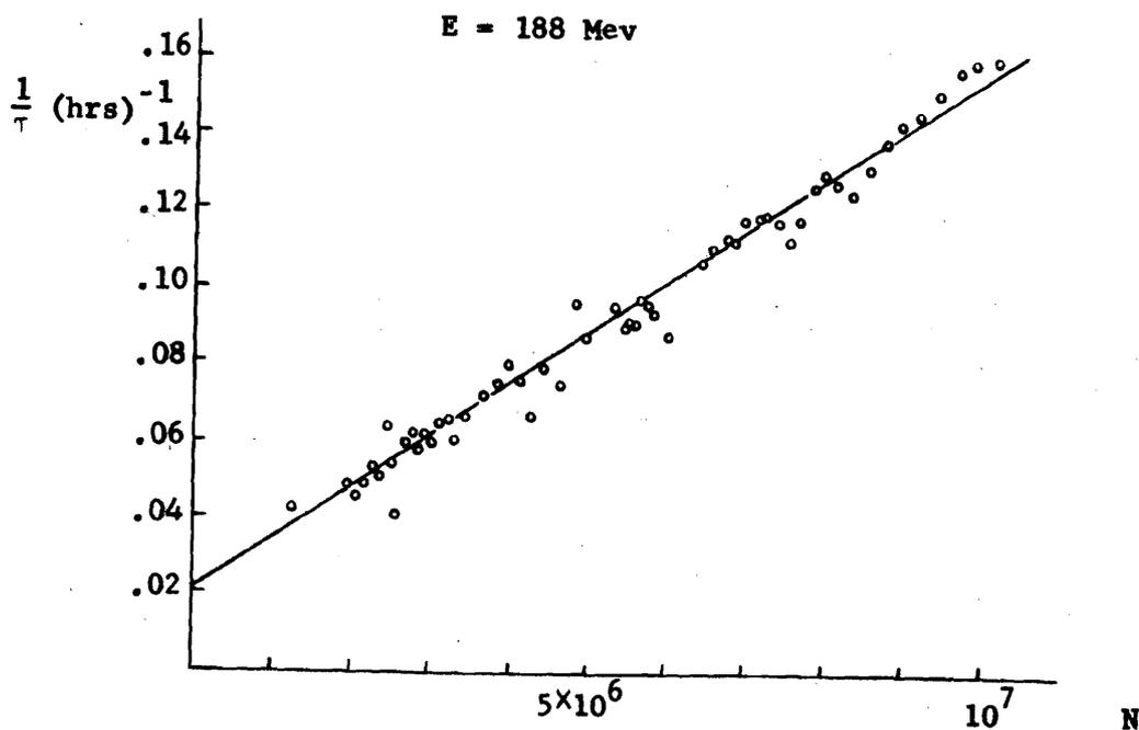
Fig. 12 - Lifetime  $\tau$  vs  $N$ , the number of stored particles in a beam, at the energy of 188 Mev
