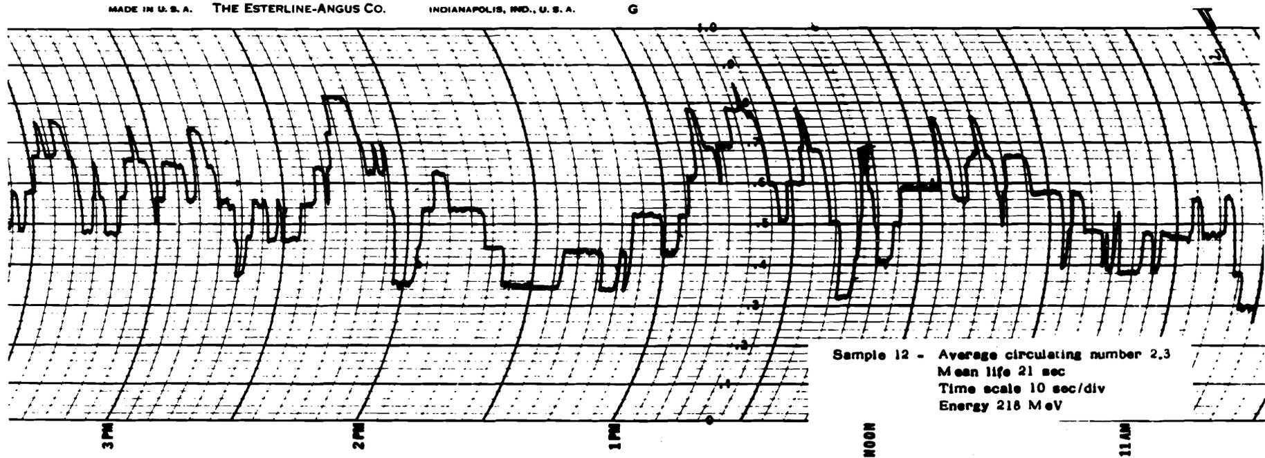
Fig. 5 - Output of photomultiplier observing synchrotron radiation from captured electrons
