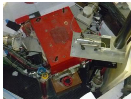
Figure 2: Top view of the separator magnet (in red) in the dedicated room. Beam is coming from the top left corner of the figure.
