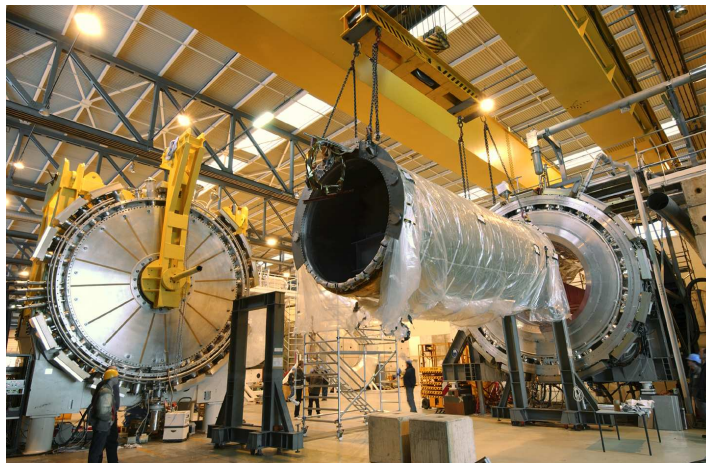
Figure 3.14: The Central Solenoid before the installation [19]. The 4 tonne coil contains 10 km of superconducting cable which is cooled with liquid helium [3]. The nominal current is 8 kA during normal operation.
