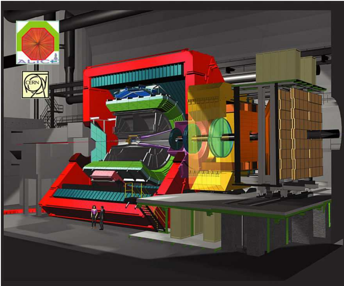
Figure 2.8: ALICE detector designed for the study of relativistic heavy ion collisions [11].
