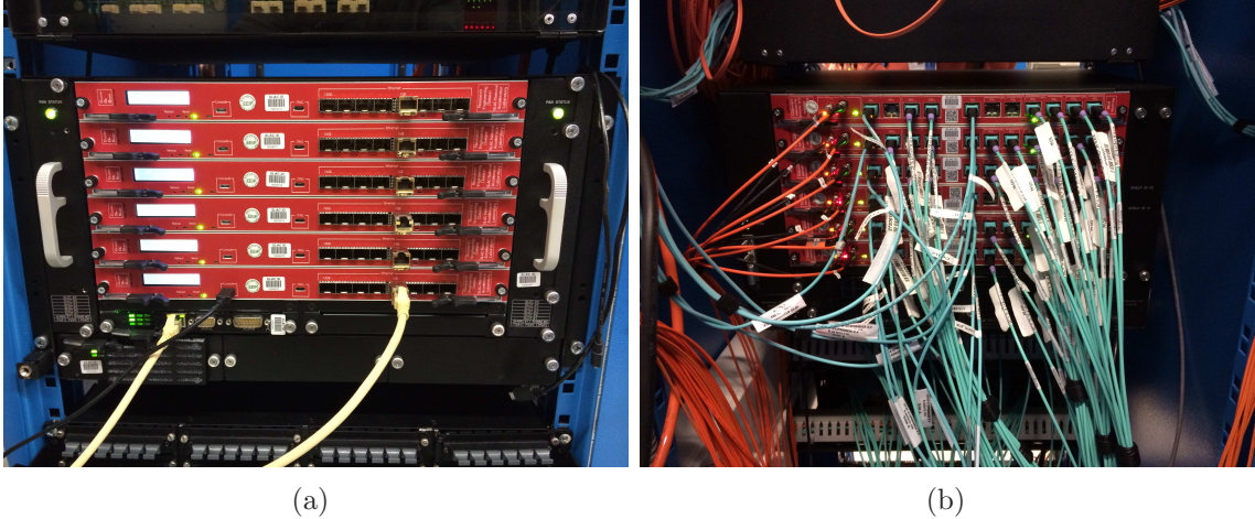
Figure 4.13: The Run-II readout system is based on boards hosted on an ATCA crate. The front view is shown in Figure (a) and the back view in Figure (b) where the RTM are hosted and the fibers are connected.
